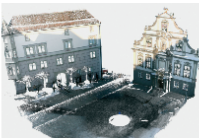
Colormapping – 3D point cloud with RGB color information
